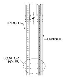
When properly assembled, both the upright label and the laminate label will remain visible during the preassembly phase. Once assembled on the bin the upright label will be covered.
