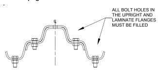
For proper orientation, ensure that the labels on the upright and laminate are both towards the bottom and that the locator holes in the middle portion of the upright and laminate line up. Bolts can be placed in these locator holes to create a pre-assembly. All locator holes, located in the middle of the upright and laminate flanges, need to be filled with bolts. These include holes in flanges that may only have one thickness of material.
