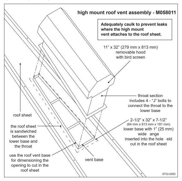
2. Evenly space all roof vents around the bin roof perimeter. Install the high mount roof vents high enough on the bin roof sheet to avoid interference with an eave ring or eave clips. Your installation may require the installation of additional roof vents at upper or intermediate roof locations (to facilitate airflow in the roof peak). Many cases require the installation of power roof vents with thermostat controls. Install the required roof vents before using the bin for the first time.
