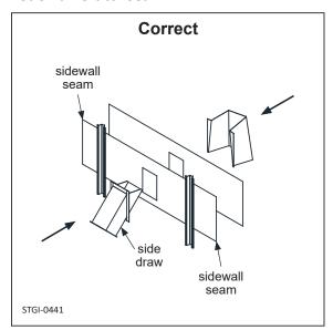
The following Figure 4 is one suggested guide for locating aeration fans and floor unload equipment.
