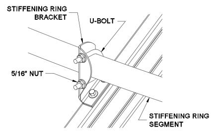
6. Once all the roof panels have been installed, make sure all nuts have been tightened.
