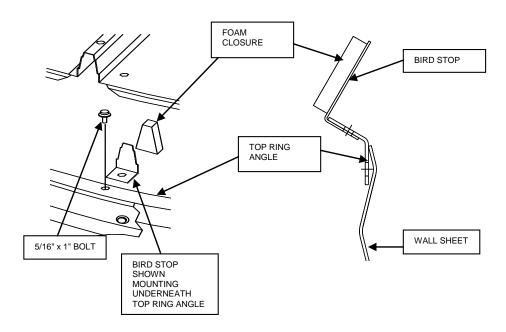
**Tip**Mounting the bird stop under the top ring angle prevents it from turning when tightening the nut.
