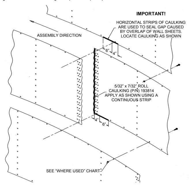
Figure 31. Wall Sheet Caulking Detail (inside view) — Metric
