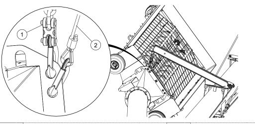
1 safety chain and hook 2 winch cable and hook
