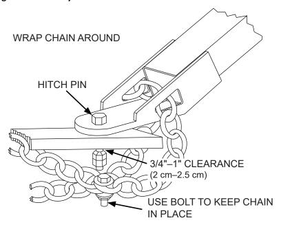
Figure 13. Hopper in Transport Position
