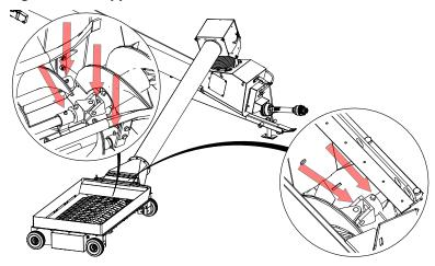
Figure 29. Upper Flighting Bearing Grease Point
