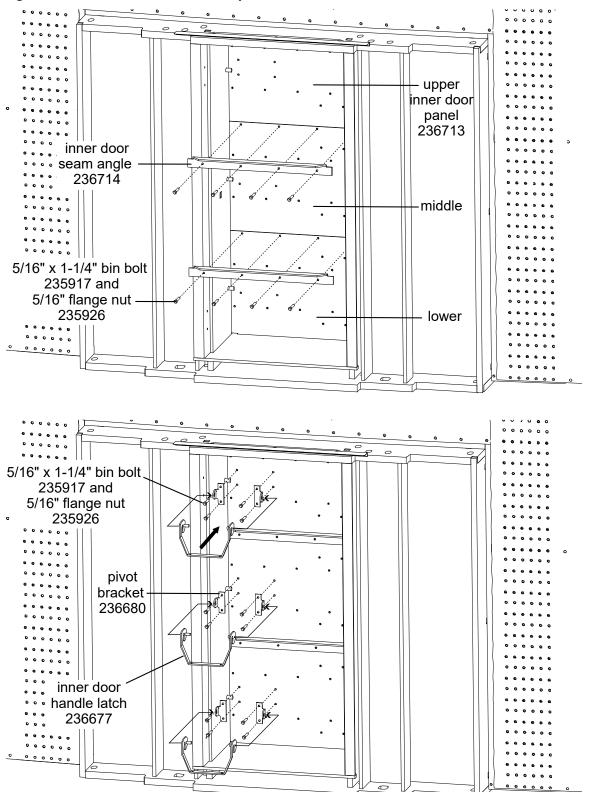
Figure 7. Inner Door Panels Assembly
