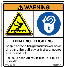
1002303-1 Rotating Flight Hazard Apply to Outside of Bin or Storage Structure
